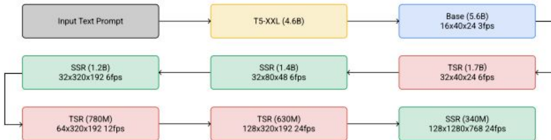
Figure 6: The cascaded sampling pipeline starting from a text prompt input to generating a 5.3-second, 1280 \times 768 video at 24fps. “SSR” and “TSR” denote spatial and temporal super-resolution respectively, and videos are labeled as frames \times width \times height. In practice, the text embeddings are injected into all models, not just the base model.
